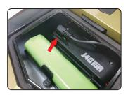
E: Plug battery DC connector into power socket in receiver box. Now boat LED navigation lights come on. Transmitter emit "Di Di" sound, transmitter two LED lights change to solid on. That means radio automatically bind with boat.
